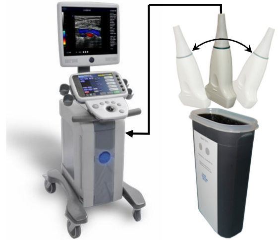
Fig. 2. The idea of SC technique used in this study. The imaging plane changes through mechanically turning the probe.
